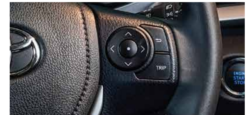
MID CONTROL SWITCHES
